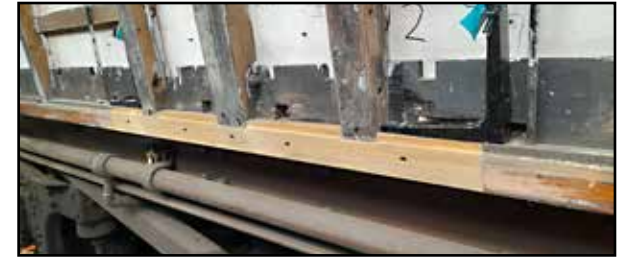
With a panel removed on TTO 56856, new hardwood has been spliced in on the bottom rail. Photo: Marcus Woodcock.
