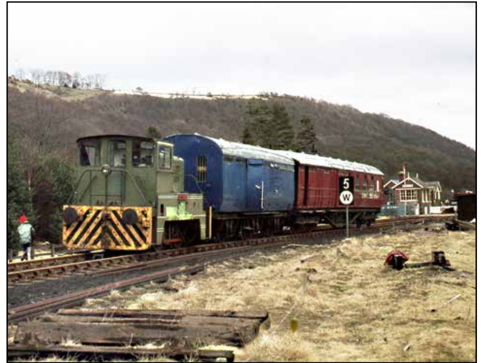
The BZ (Brake 6-wheeled) 70687, is on York Area Group p.way duty, along with the mess coach, ADE 320421, formerly BCK 10178. Sadly, the condition of the BZ deteriorated until it was beyond repair - except for the underframe which now lives on under GER No. 8 (left). Photo: Nick Carter.
