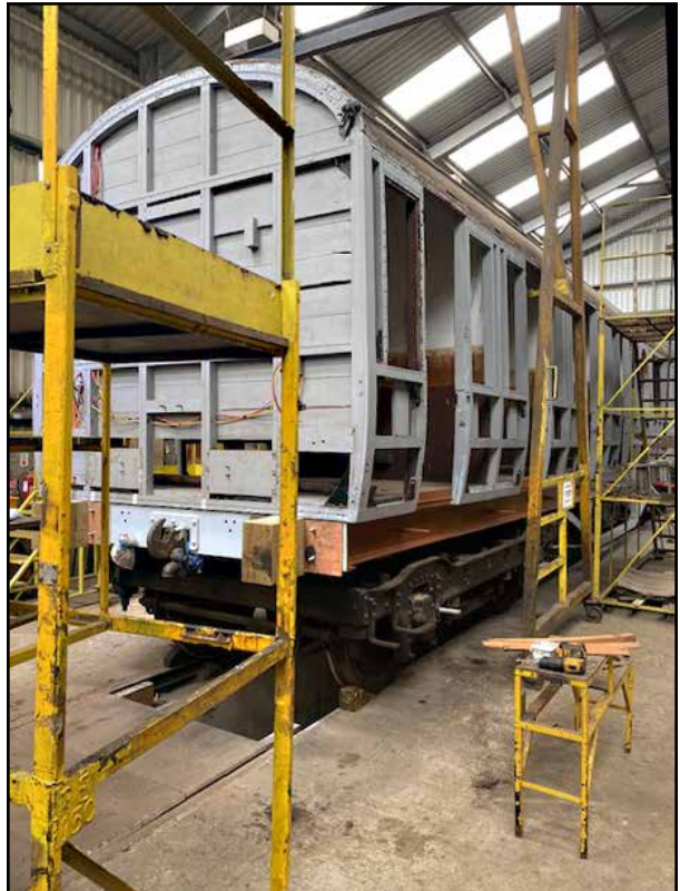
Third Corridor (TK) 23896 is coming along well inside Unit 10, Kirby Misperton under the stewardship of Andrew Daniel. Refurbished teak panels are being fitted, as this view taken on June 11 illustrates. Photo: Murray Brown.
